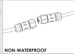
Leaving the connectors unprotected or disconnected may cause water infiltrations and consequent product malfunctioning.
