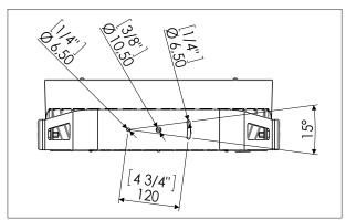
Use the holes  $\varnothing 10.5$  (3/8") or  $\varnothing 6.5$  (1/4") in the bracket to fix the unit.
