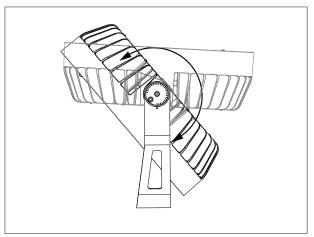
2. Rotate the bodies of the unit towards desired direction and tighten the screw "1".
